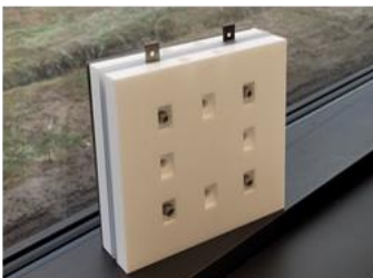
Figure 4.7.2: The PV-integrated electrolyzer realized, with a) the CIGS PV module or test illumination, b) the 20cm by 20 cm newly designed electrolyzer element, and c) the completed assembly
