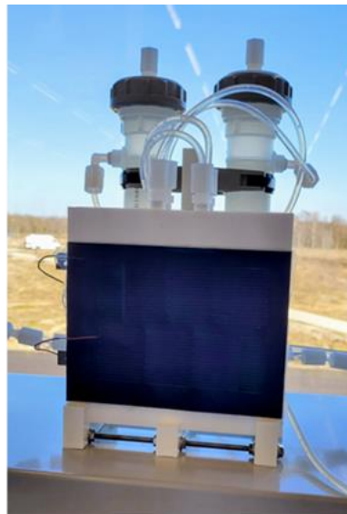
Figure 4.7.2: The PV-integrated electrolyzer realized, with a) the CIGS PV module or test illumination, b) the 20cm by 20 cm newly designed electrolyzer element, and c) the completed assembly
